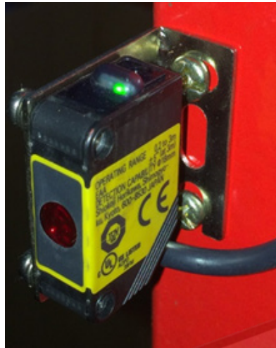
Power on but not aligned
